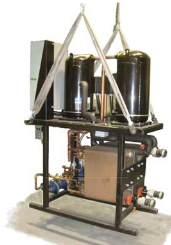
Figure B: Lifting from above
