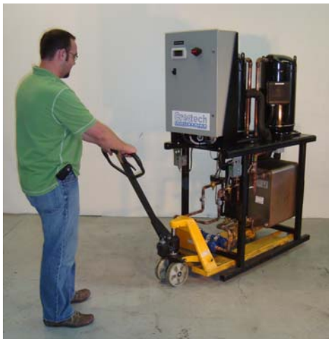
Figure A: Lifting from below
